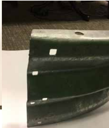
Full depth corrugation with standard end.
